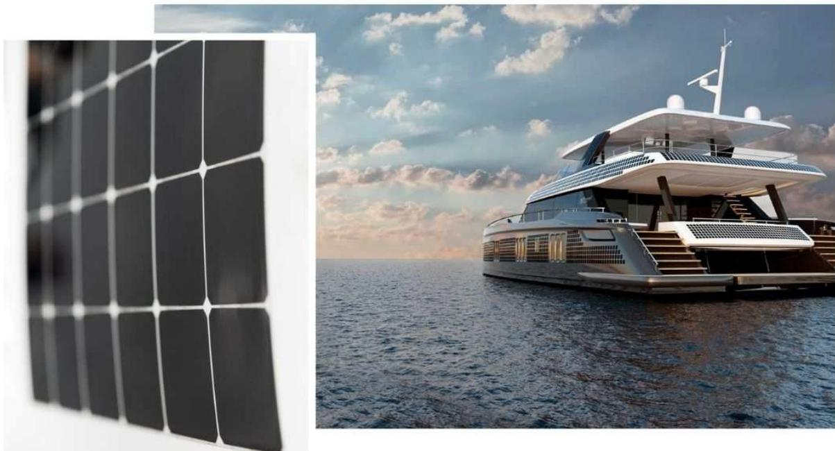
The shipyard’s solar skin system is currently being integrated on both power and sail catamarans within the Sunreef Yachts Eco range of luxury catamarans. The panels are entirely flush with all curved composite structures including masts, hull sides and biminis. With maximized solar power, the Sunreef Yachts Eco deliver the industry’s top solar power efficiency.
